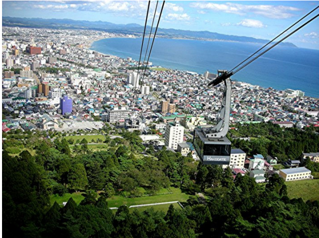
Left: Hakodate city and the Pacific Ocean to the east. A matching tram car descends past us and helps pull our gondola up the mountain.
